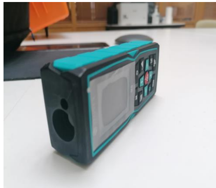
Figure 4. Laser rangefinder Stonex M6 used in the study (source: author's photo fixation)
