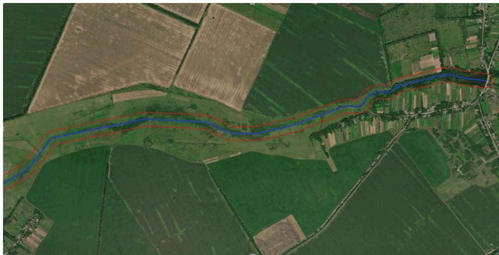
Fig. 1. River vector with a constructed buffer of the 100 m coastal protection zone.
